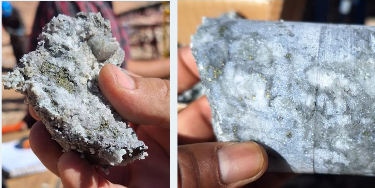
Drillhole DDH-PO-01. Sphalerite mineralization
