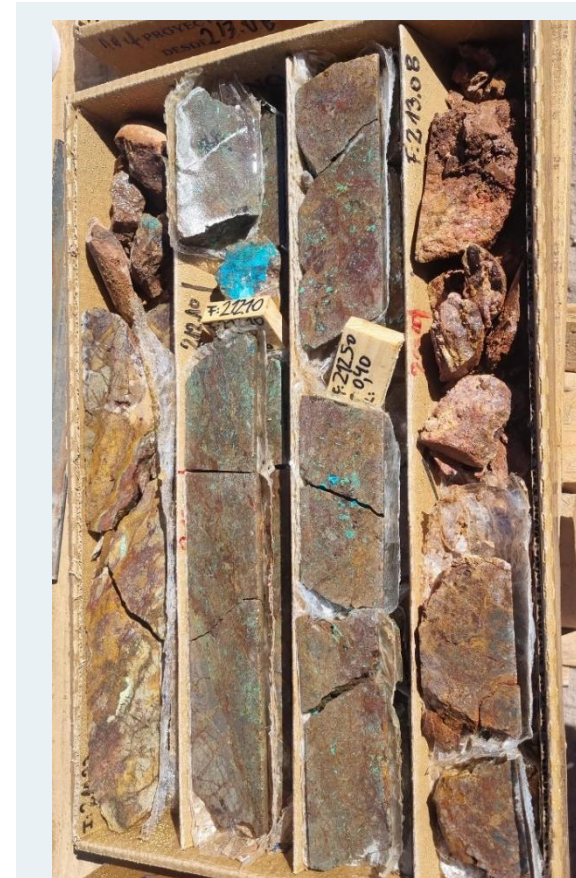
Drillhole DDH-PO-02. Copper Oxides (Chrysocholla, Limonites, Brochantite)
