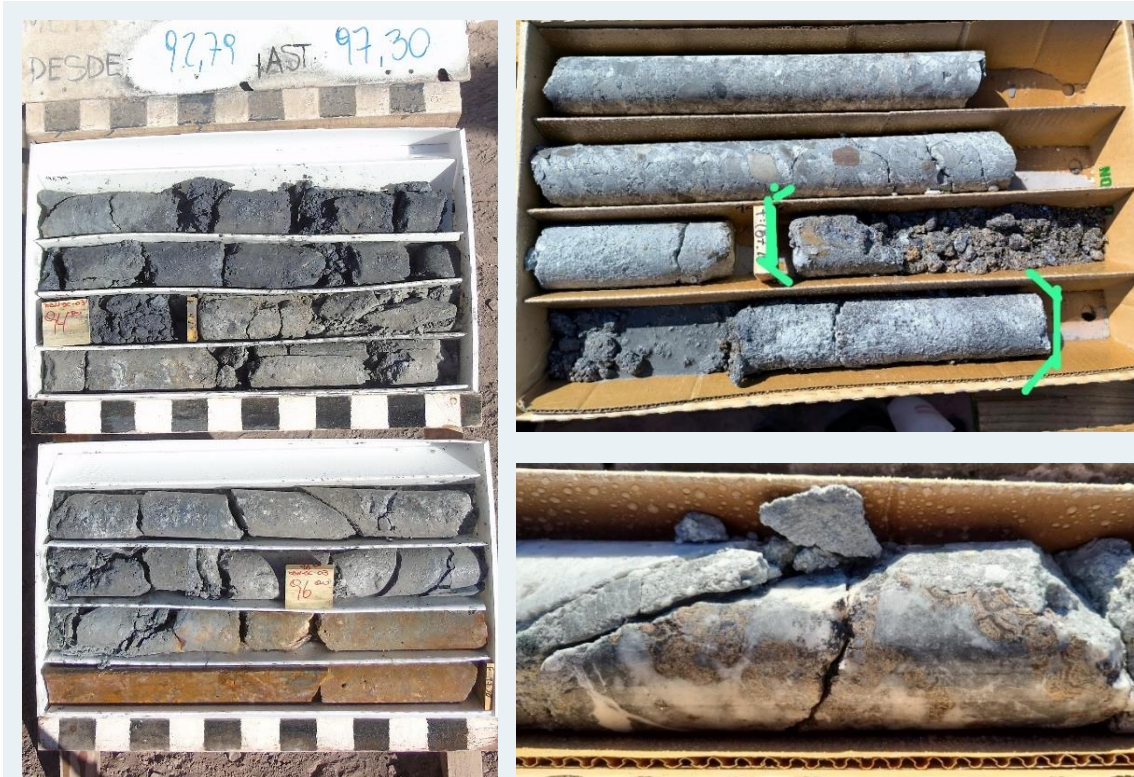
Semimassive and Qz-breccia polymetallic sulphides, including 26%Zn+270g/t Ag + 7% Pb+ 0,15% Cu intercept
