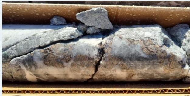
Semimassive and Qz-breccia polymetallic sulphides, including 26%Zn+270g/t Ag + 7% Pb+ 0,15% Cu intercept
