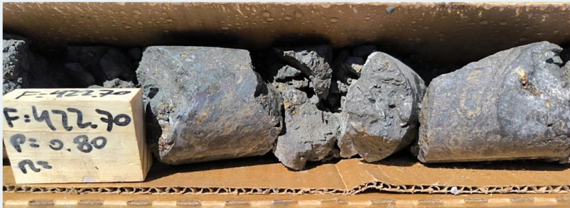
Drillhole DDH-PO-01. Sphalerite mineralization
